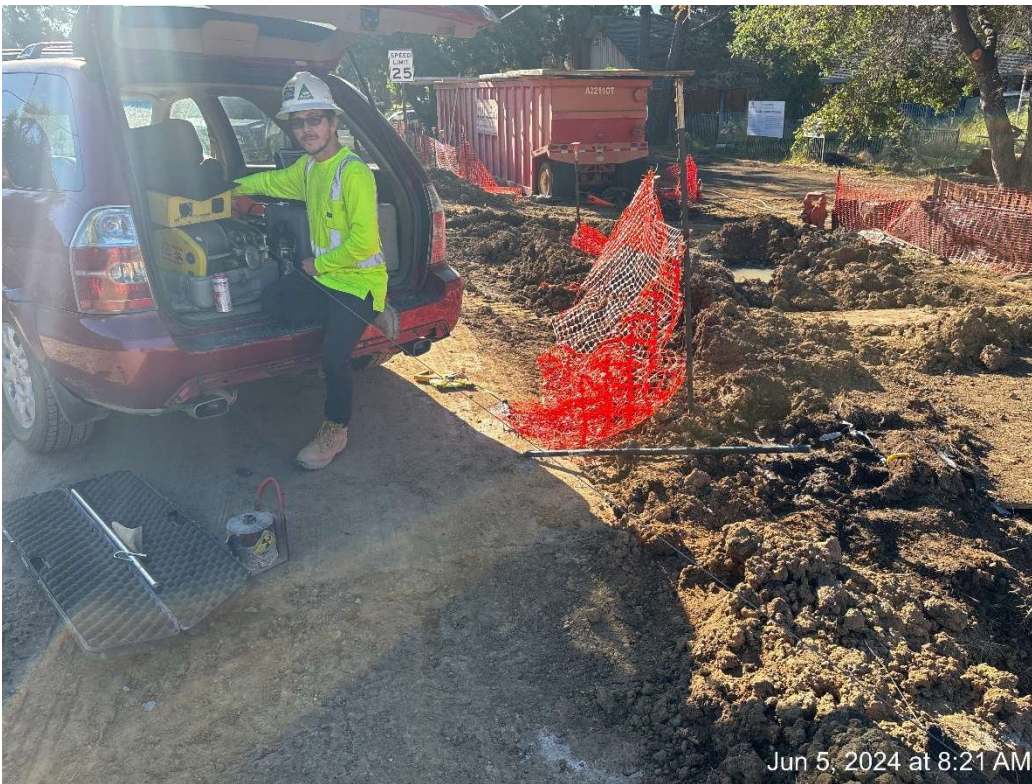
Figure 1 – ACS performing Gamma Gamma Logging (CT-233) of CIDH Piles.
