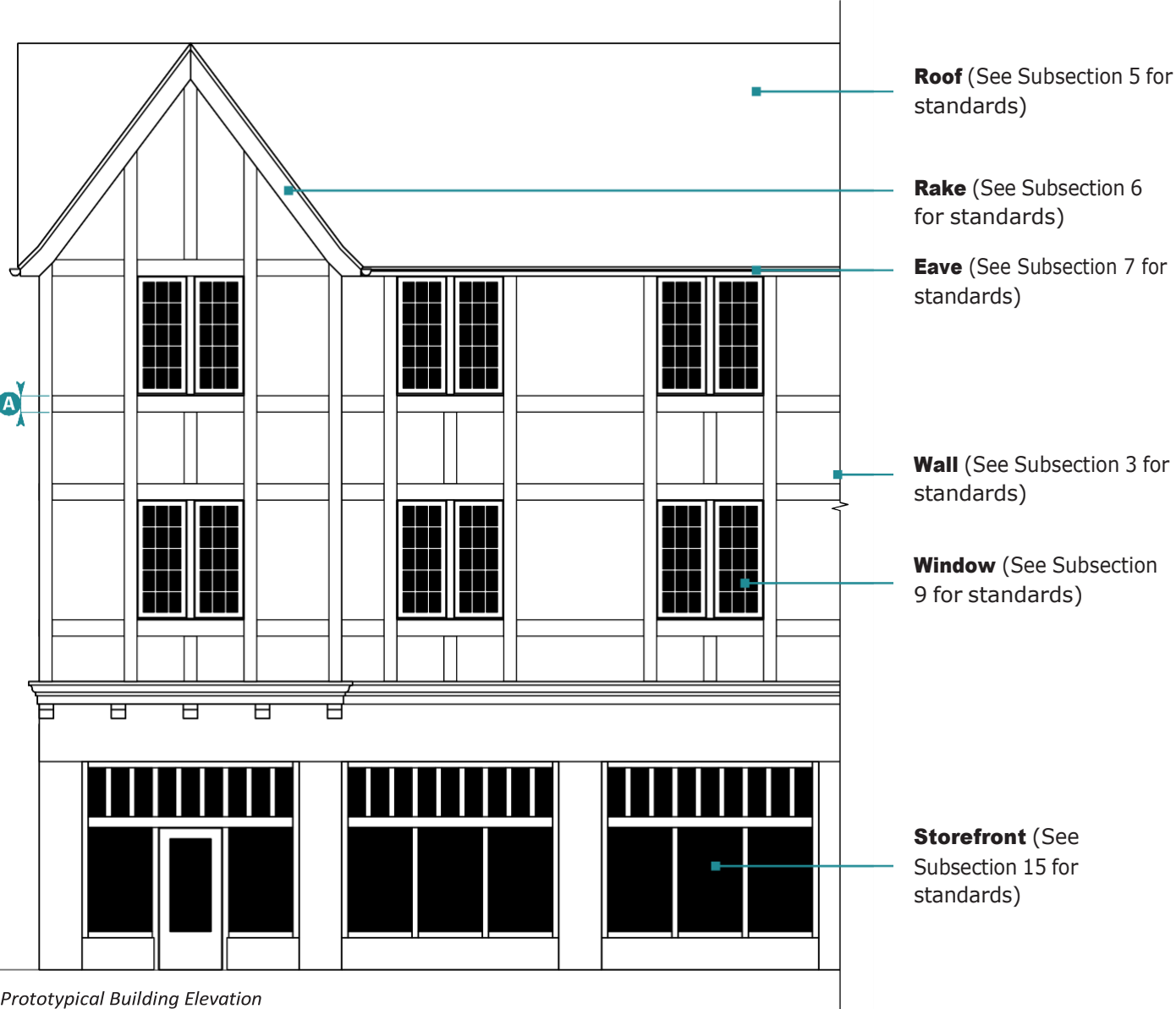
Prototypical Building Elevation
