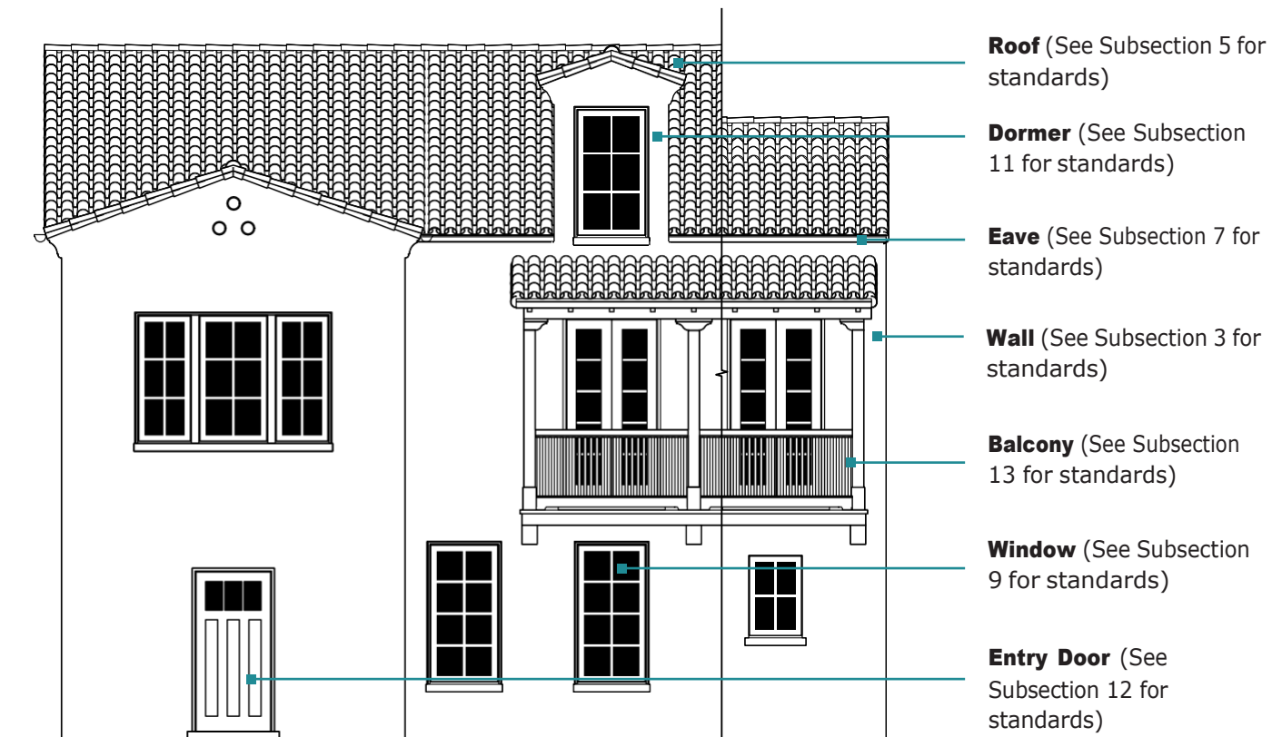
Prototypical Building Elevation
