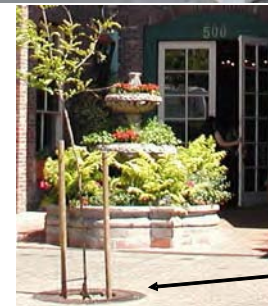
tree grate facilitates foot traffic
