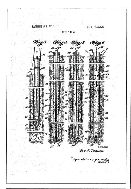
For pipelines, anodes are arranged in groundbeds either distributed or in a deep vertical hole depending on several design and field condition factors including current distribution requirements.
